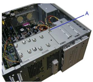
Figure 4 - 9 : Replacing the Screw
